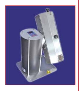
The bottle shaker LAB.SHAKE is an overhead turning device for glass and PET bottles of the beverage industry.
