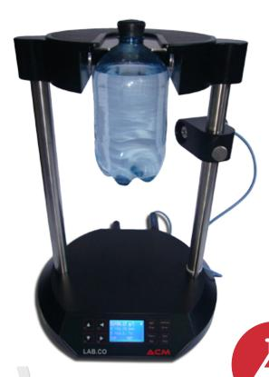
Laboratory CO<sub>2</sub>-Meter **LAB.CO** for non-invasive high precision dissolved CO<sub>2</sub> content measurement in bottled beverages.
